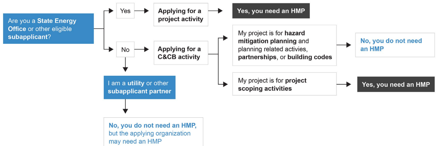
Figure 3: Hazard Mitigation Plan Requirement Decision Tree
